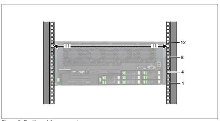
Figure 5: Position of the cage nuts
